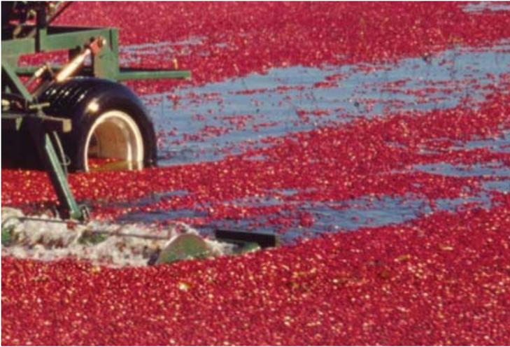
A water reel harvester at work in a cranberry bed that has been flooded for harvest.
